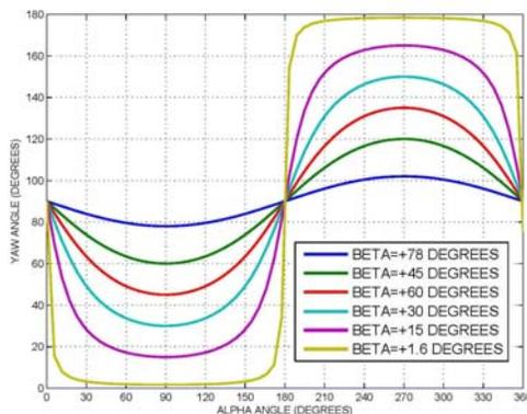
**Figure 10. SNP Yaw Angle vs. Orbit Alpha, for Positive Beta Values**
