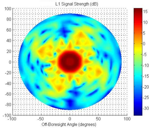
**Figure 16. Average Improved Antenna Pattern - L1, 3-D Plot**
