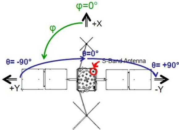
Figure 7. Antenna Orientation Angles: Around Boresight (phi,  $\phi$ ) and Off-Boresight (theta,  $\theta$ )
