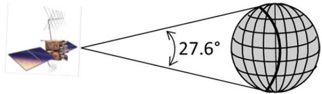
Figure 2. Earth Terrestrial Service Volume Definition
