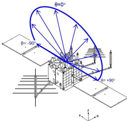
Figure 8. Antenna Orientation - Off-Boresight, Side View
