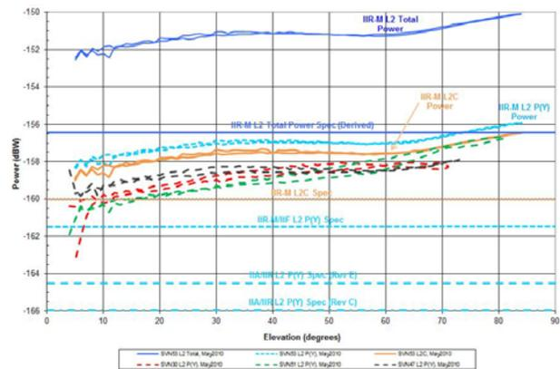
Figure 13. Code Power Measurements - L2
