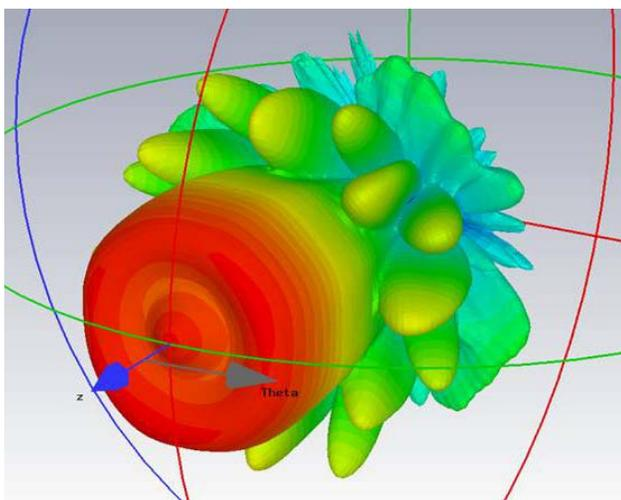
**Figure 21. Notional GPS Signal Transmit Pattern with Sidelobes (from [42])**
