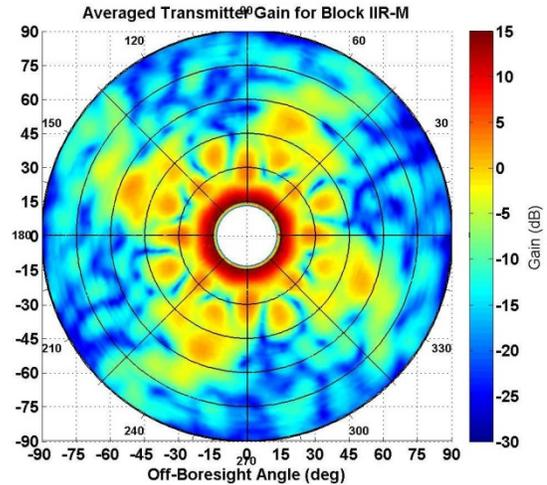
**Figure 19. ACE Measurement of the Average GPS Block IIR-M Antenna Signal [18]**
