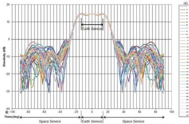
**Figure 18. Average Improved Antenna Pattern - L2**
