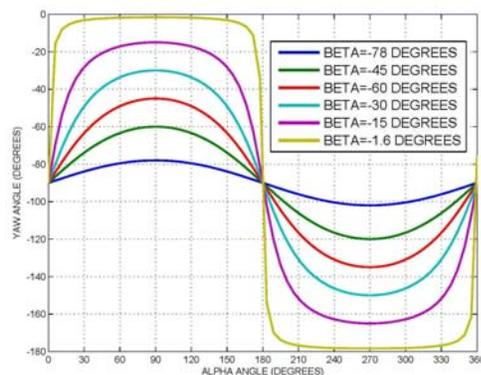
**Figure 11. SNP Yaw Angle vs. Orbit Alpha, for Negative Beta Values**
