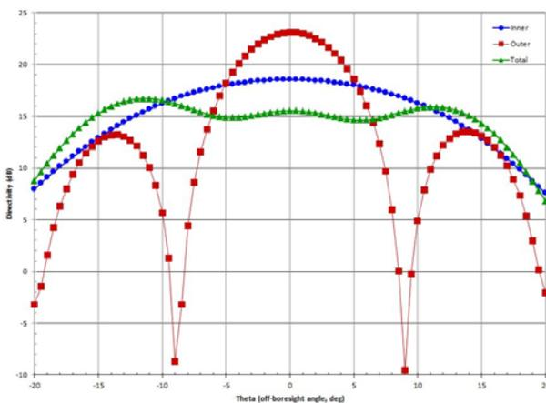
**Figure 5. Nominal Antenna Panel Pattern from Inner and Outer Rings**
