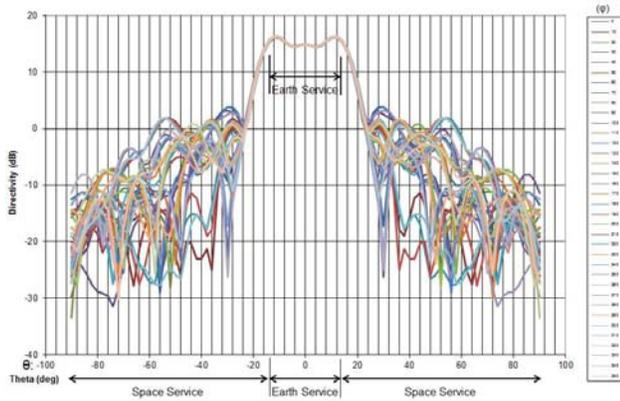
**Figure 15. Average Improved Antenna Pattern - L1**
