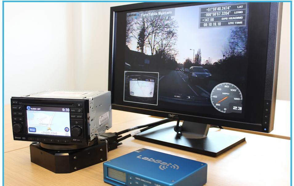
**RECORD** real world GNSS signals, vehicle dynamics and live video
