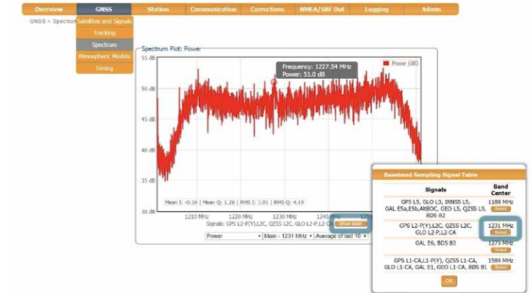
Figure 7 – Visualising RF interference – the spectrum view plot
