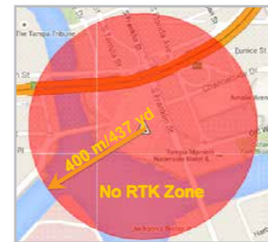
Figure 13 – 10 mW Chirp jammer without mitigation
