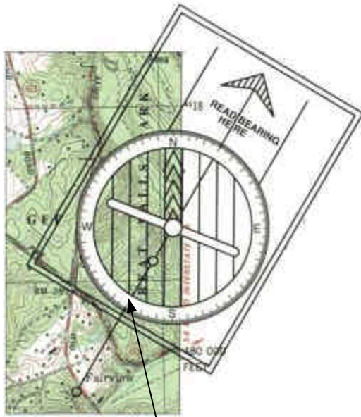
This is the bearing of the line.
